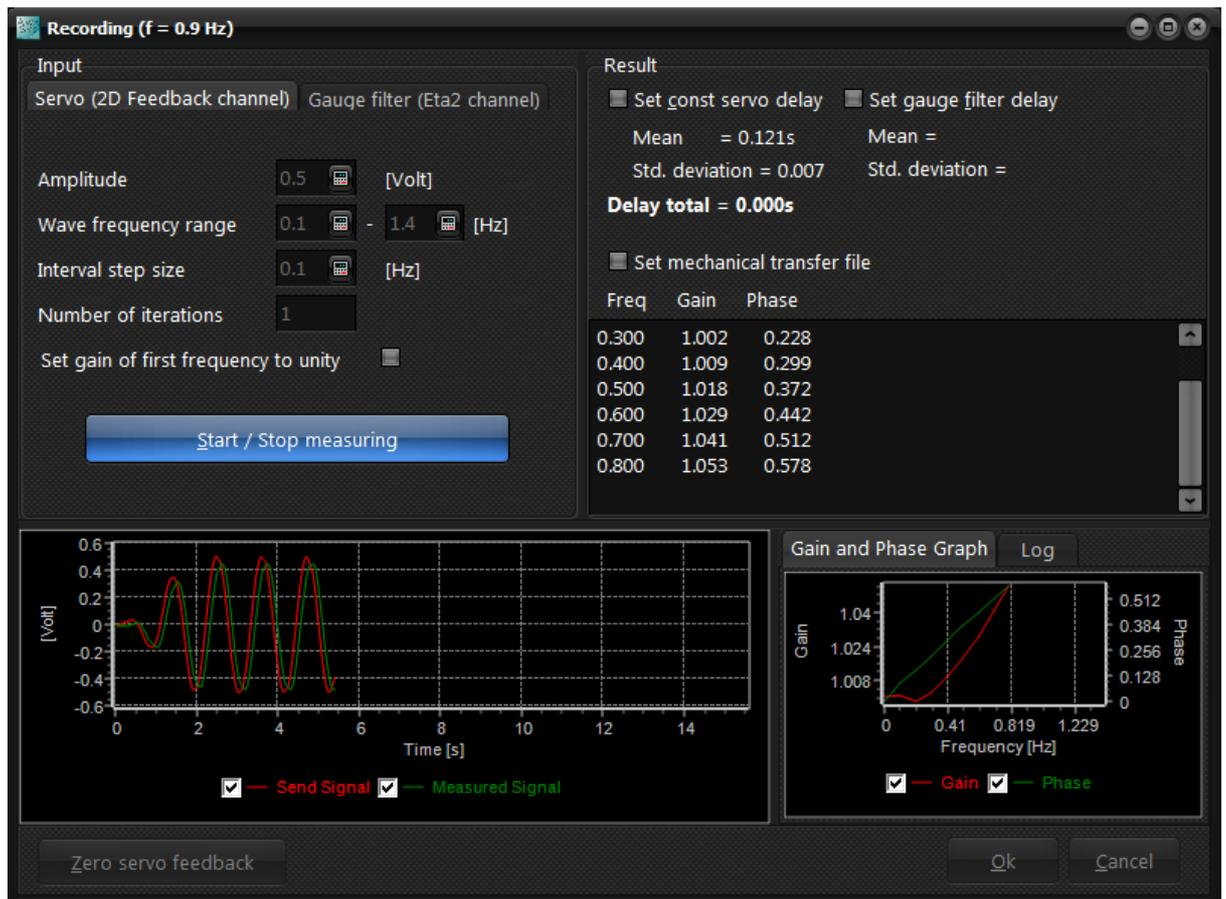
Absorption performance can be improved by compensation of a possible delay. This dialog can measure the delay and performance of the wave generator and hereby automate the process of creating a mechanical transfer file. The dialog can also measure a delay introduced by sending the wave gauge signal through a filter.
