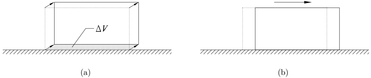
Figure 13: Mechanisms corresponding to associated (a) and nonassociated (b) flow rules.
